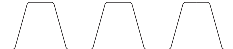
Figure 3.2 T837 100Hz VCO Control Line Wave Form
